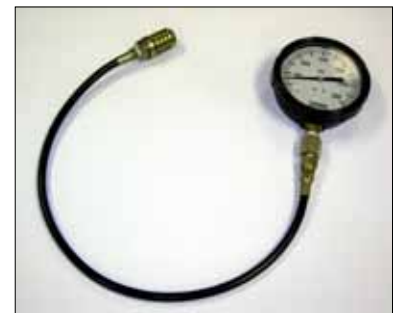
Hydraulic test gauge w/connector 3000 psi range, p/n 56504516
