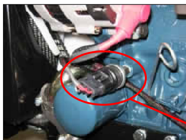
Oil Pressure Sensor (above oil filter)
