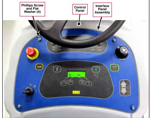
3. Carefully lift the Interface Panel Assembly out of the Control Panel.
