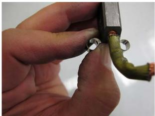
d. Push brush back against the spring and insert a stiff temporary retaining wire (Paper clip) through the access hole in the end cover. (Remove silicone sealer from the holes) The wire must go through the holes in the brush holder just in front of the brush to hold the brush back against the spring pressure.
