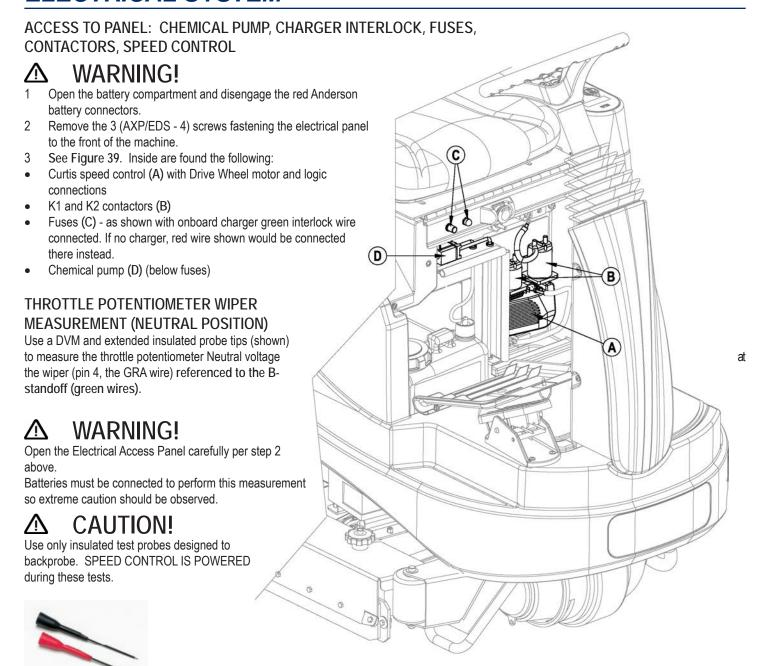
Referenced to the negative battery standoff, the wiper voltage should read:
