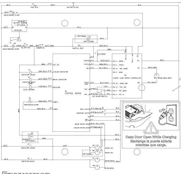
NOTES:  $\underline{\Lambda}$  DISCONNECT RED WIRE ON CB2 AND REPLACE WITH GREEN WIRE FROM CHARGER WHEN ON BOARD CHARGER IS USED
