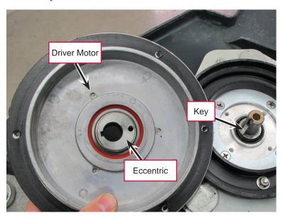
6. Note the orientation of the brush motor electrical leads relative to the deck to make sure you install the motor in the same position. You may want to mark the orientation of the brush motor to the motor plate. Then separate the brush motor from the motor plate by removing the 4 attaching screws and remove the motor.
