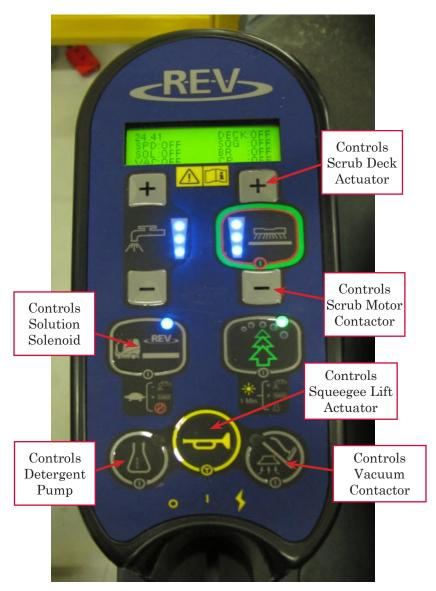
Service Test Mode Switch Operation
