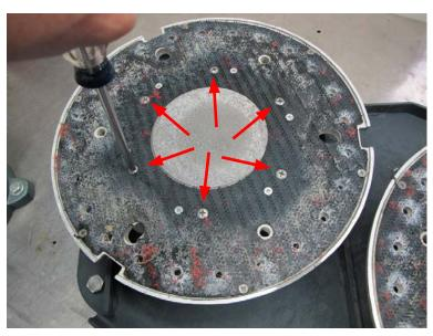
4. Remove the counter weight by removing the two attaching bolts
