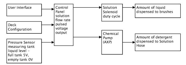
A malfunction of either the Pressure Sensor, the Control Panel, or an air leak in the pressure sensing system may affect the performance of either the Chemical Pump or the Solution Solenoid, or both.
