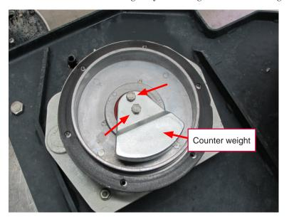
5. Lift the driver motor with the eccentric from the brush motor shaft being careful not to lose the square-cut key.
