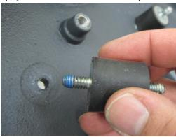
2. Install the isolators in the brush head. Position each one so that the color stripe it will be visible when the motor plate is installed. Torque each nut to 8-10 ft. lbs. (10.8- 13.5 N m). Install the 4 plastic covers over the nuts.
