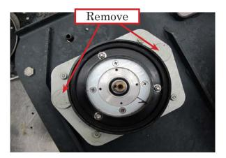
4. Remove the motor plate by removing the 4 isolator nuts. Inspect the splash shield and replace if damaged...
