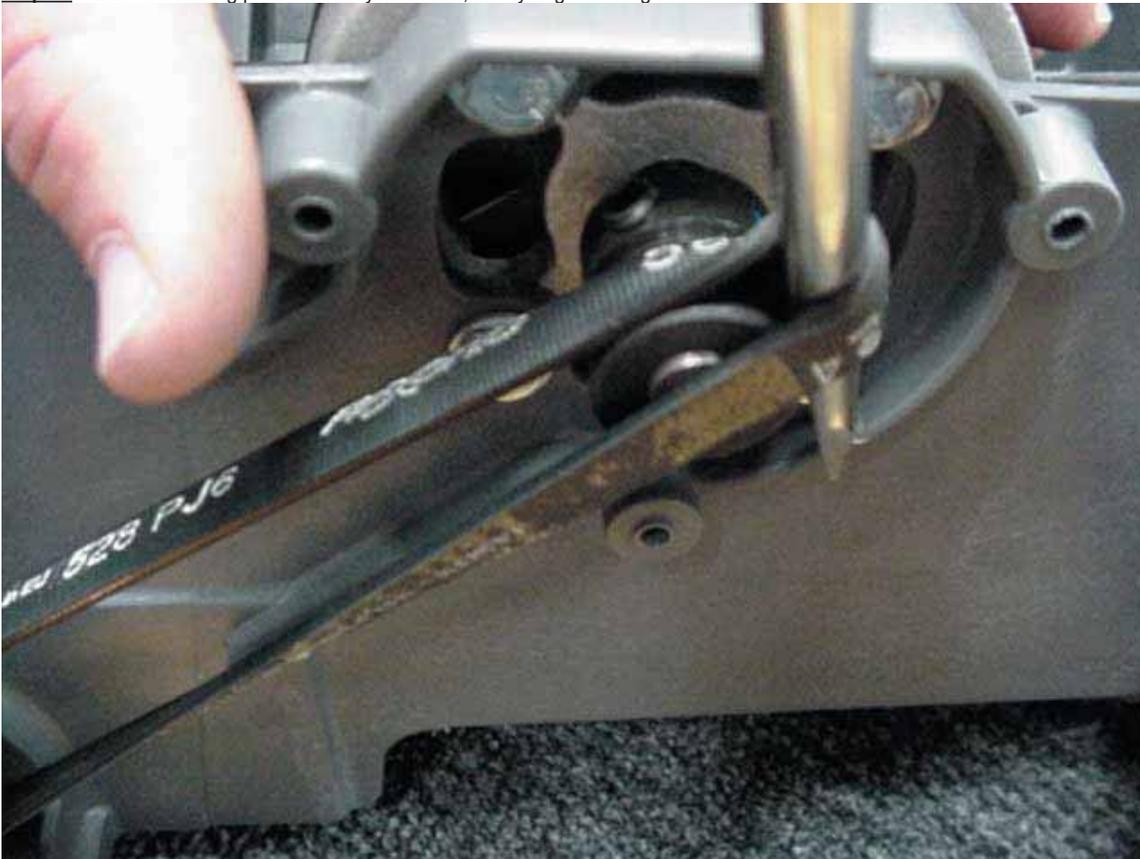
**Step 4:** Continue rotating until screwdriver tip clears the belt and the belt rests on the sheave.
