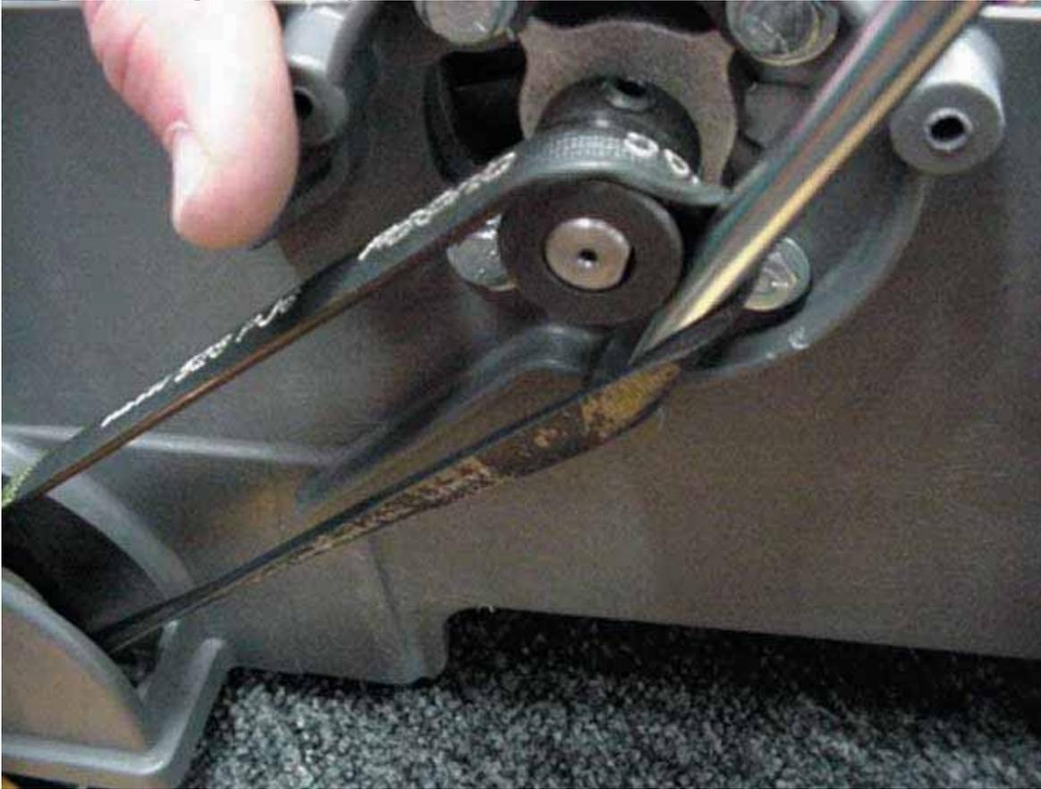
**Step 5:** Although the belt may be on the sheave, it's possible that it is not on properly as shown below. Inspect the belt to make sure it is completely on the sheave.
