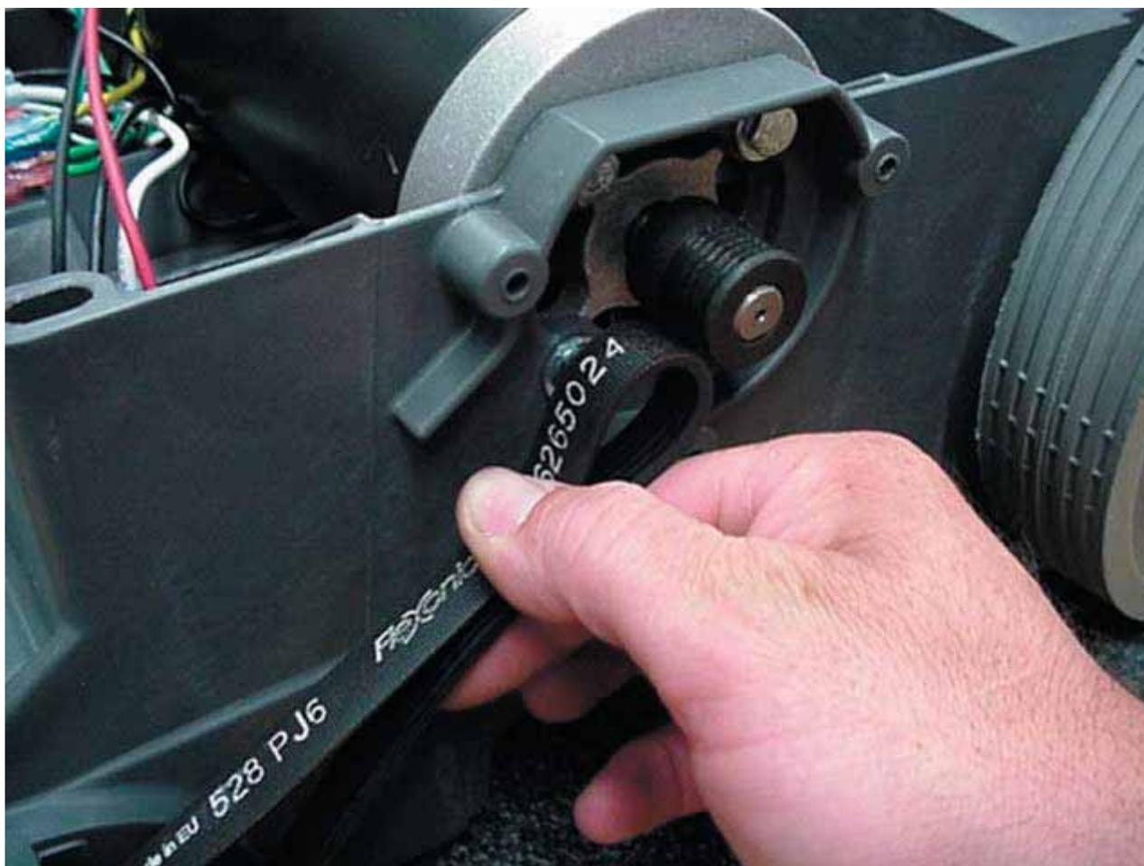
**Step 2:** Place a large regular screwdriver through belt and up against sheave on brush motor. It is important that the tip of the screwdriver be placed on the sheave. This will prevent the screwdriver from rotating and also prevent the screwdriver from scratching the base when it is rotated. Use your thumb to put pressure on the belt as shown below.
