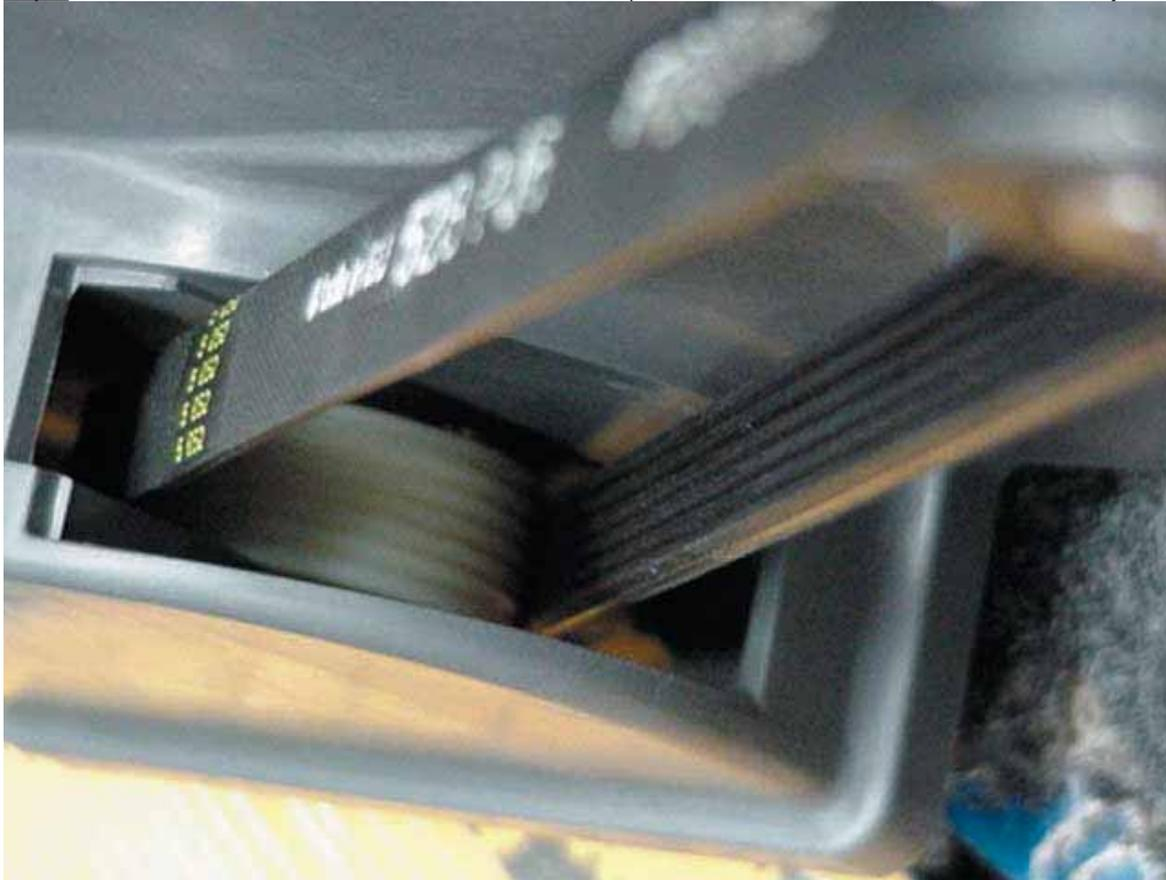
**Finish:** Reinstall belt cover, pulley clip, and brush. If the solution hose has been removed to provide more room, reattach it to solution tank. Reattach solution tank to base. If handle brackets were removed to provide more room, reattach handle to brackets.
