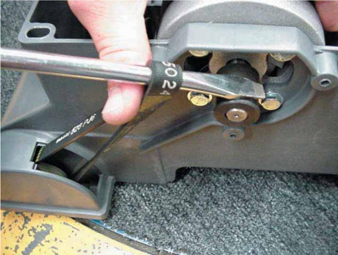
**Step 3:** While maintaining pressure with your thumb, slowly begin rotating screwdriver about the sheave as shown below.
