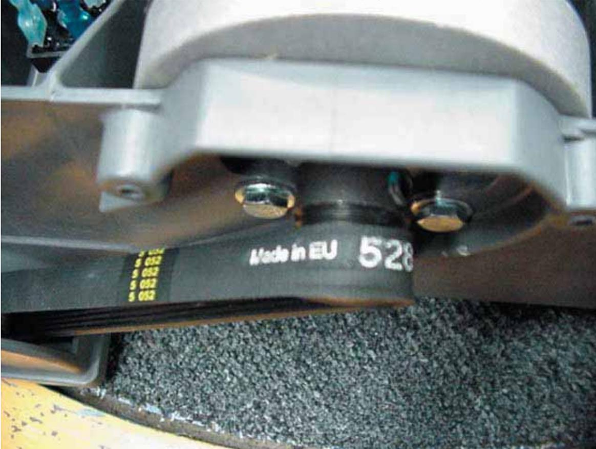
**Step 6:** If necessary, rotate the belt until it squares itself on the sheave as shown below.
