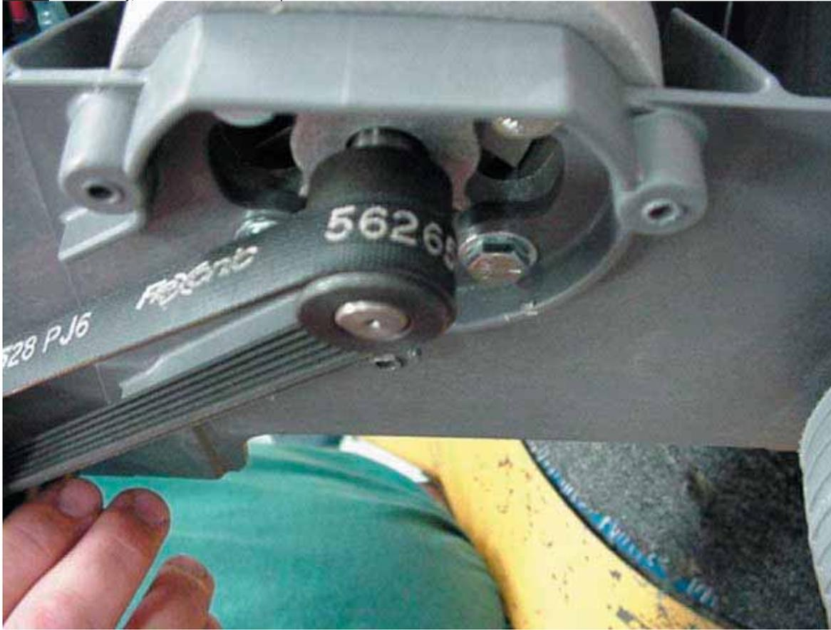
**Step 7:** Look down at the brush drive sheave to make sure the belt is square on this sheave as well. If not, continue to manually rotate the belt until it is.
